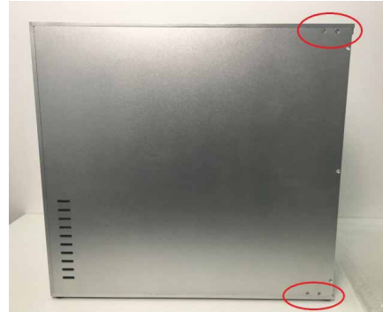
Data acquisition system side panel fixing screws
