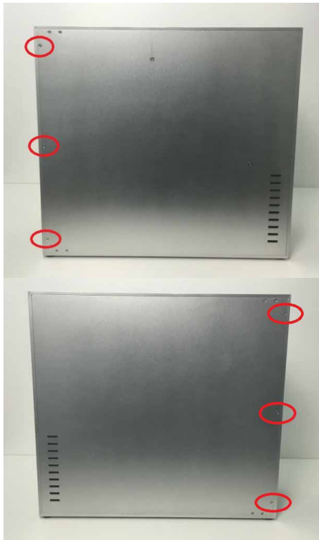
Rear panel fixing screws of data acquisition system
